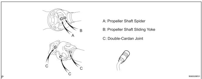
(b) Tighten the bolts of the propeller shaft.
